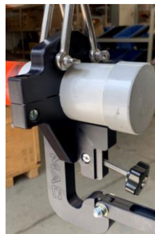
Insulator Installed with Conductor Holder Open
