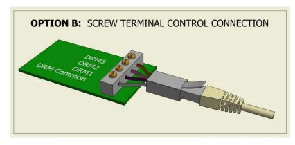
The RJ45 Adapter Cable is used to connect the TMAC DCSR to air conditioners fitted with SCREW terminals as the DRM connection. The table below shows which coloured cable must be connected to each DRM terminal.
