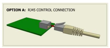
The TMAC DCSR CONTROL CABLE is connected to the dedicated DRM connector on the air conditioner. The connector will either be an RJ45 connector (OPTION A), or a set of screw terminals (OPTION B).
