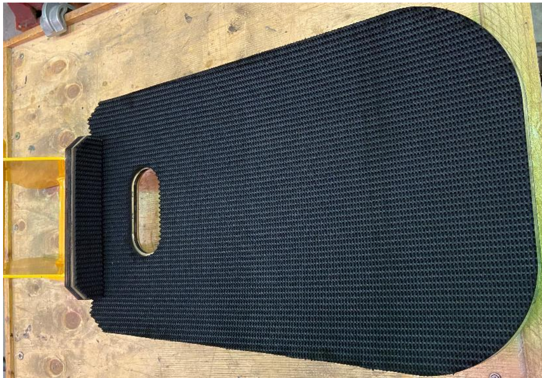
Figure 4 - Completed Replacement of Deck, Kickboard and Roughtop
