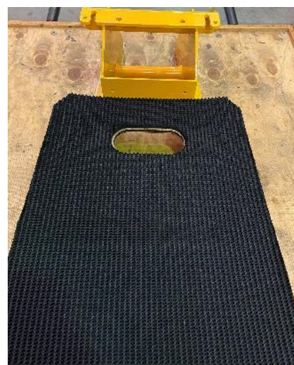
Figure 3 - Deck and Rough Top glued in Place
