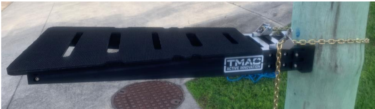
Figure 5 - Ensure Platform is Level with all Four Pads in Contact with the Pole
