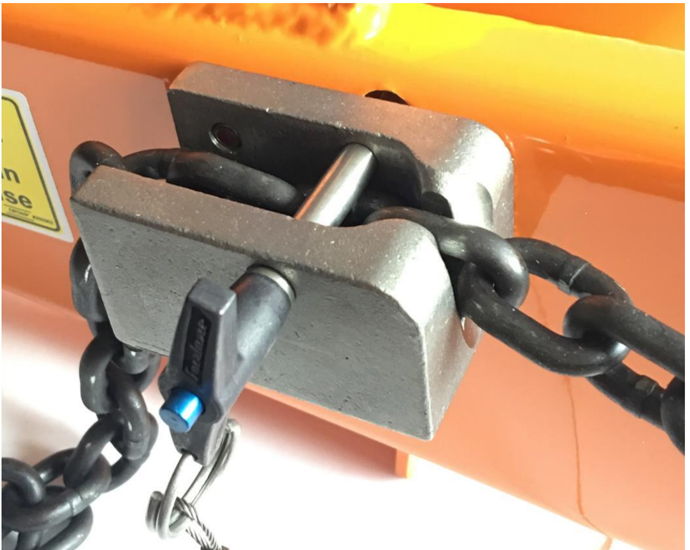
Detent pin locking chain in position
