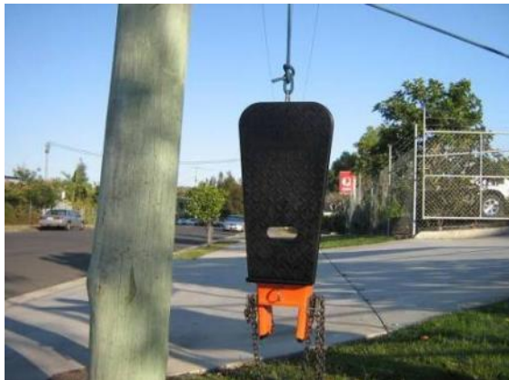
Lifting with rear "U" bolt
