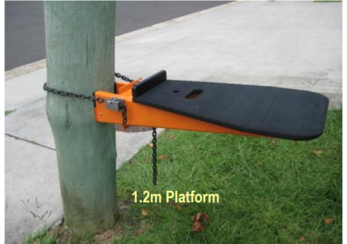
1.2m Platform all four pads in contact with pole
